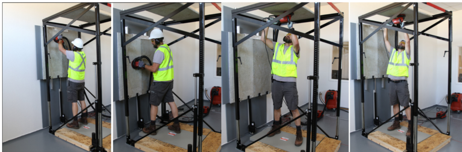
Figure 4. Adjustable height ceiling and wall apparatus (at UCSF) that holds different materials (concrete, brick wall, dry wall) for tasks requiring forward reach and overhead postures.
