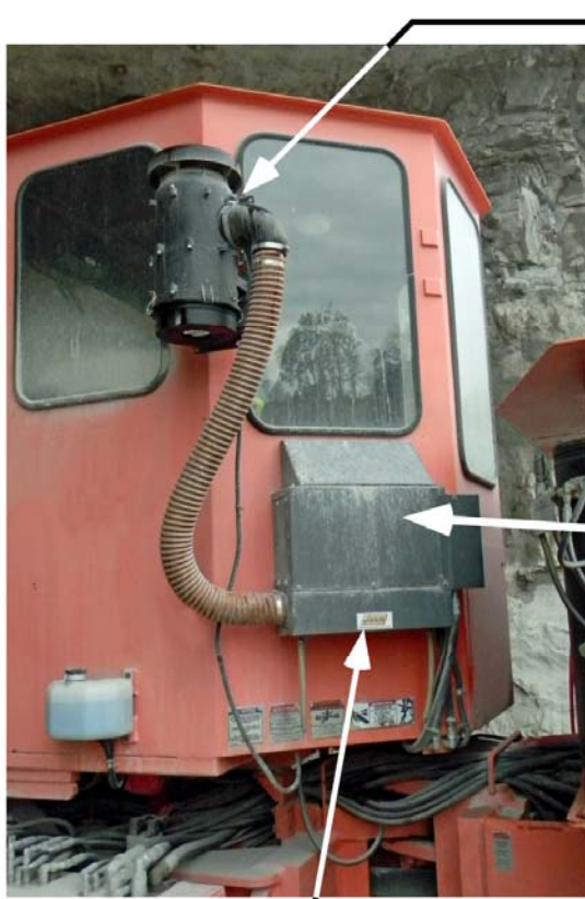
Recirculation pickup point
