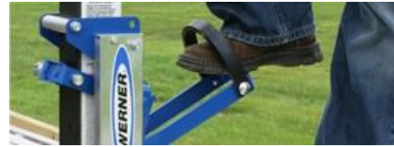
Pump Jack System
