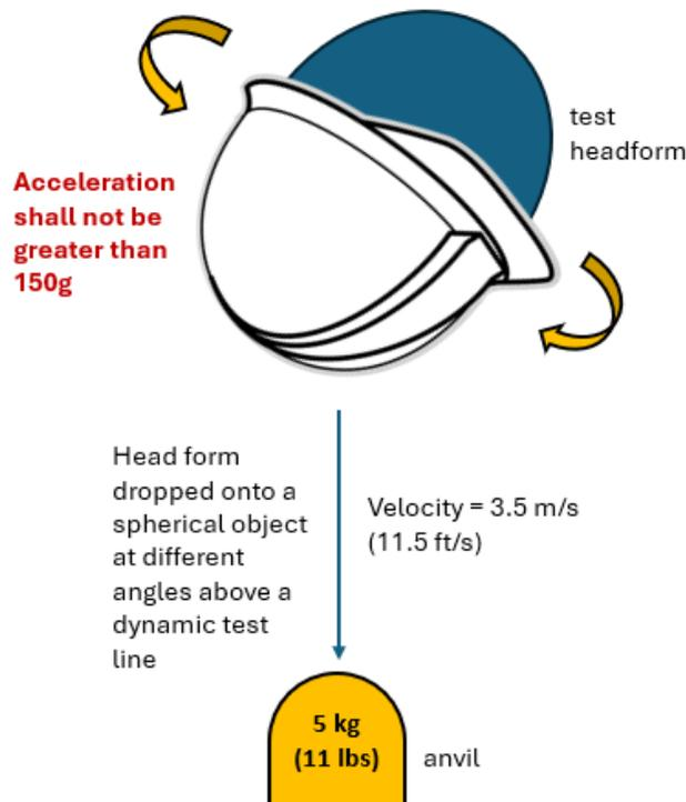
Figure 4: **TYPE II ONLY** OFF-CENTER PENETRATION TESTING
