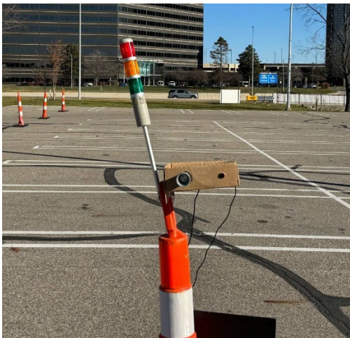
Fig. 3. The designed work zone alerting system
