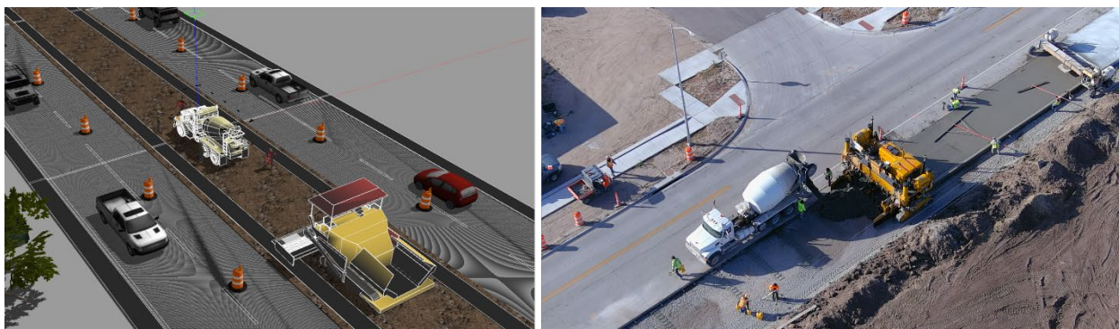
Figure 3. 3D work zone modeling in Gazebo (left) and real-world scenario (right)
